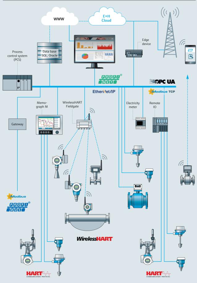
System integration with Endress+Hauser field measuring devices
