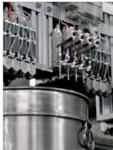
Filling process using multiple Coriolis flow meters
