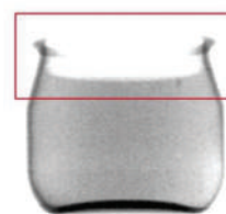
Figure 15: Yoghurt pot with low fill level
