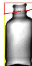
Figure 7: Detection of missing cap
