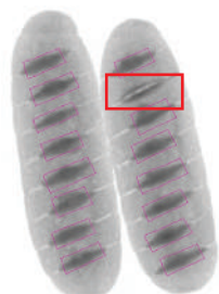
Figure 4: Shows two garlic baguettes with one low-fill
