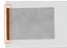
Figure 18: Wound dressing trapped within the seal
