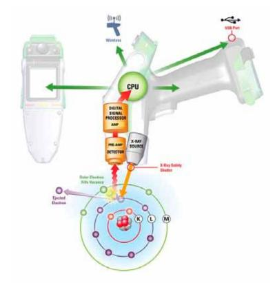
now, new handheld XRF analysers are moving this technique from the lab to the production line or field. The elemental composition of foreign bodies (down to around 0.5 mm) can be determined very easily with reliable, low-cost, lab-quality information — giving users a 'fingerprint' of the contaminant.
